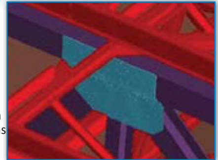
Initial Gusset Plate Failure
